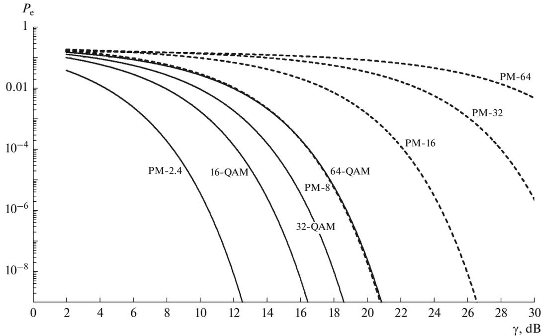
**Fig. 2.** Probabilities of bit error of coherent reception of phase-modulated signals (PM) with a constant envelope (dashed curves) and spectrally efficient signals with quadrature amplitude modulation (QAM).
