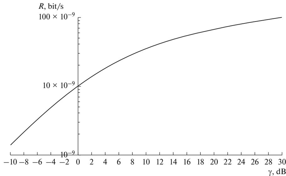
Fig. 5. Dependence of communication channel transmissivity on signal-to-noise ratio in channel band of 10 GHz.
