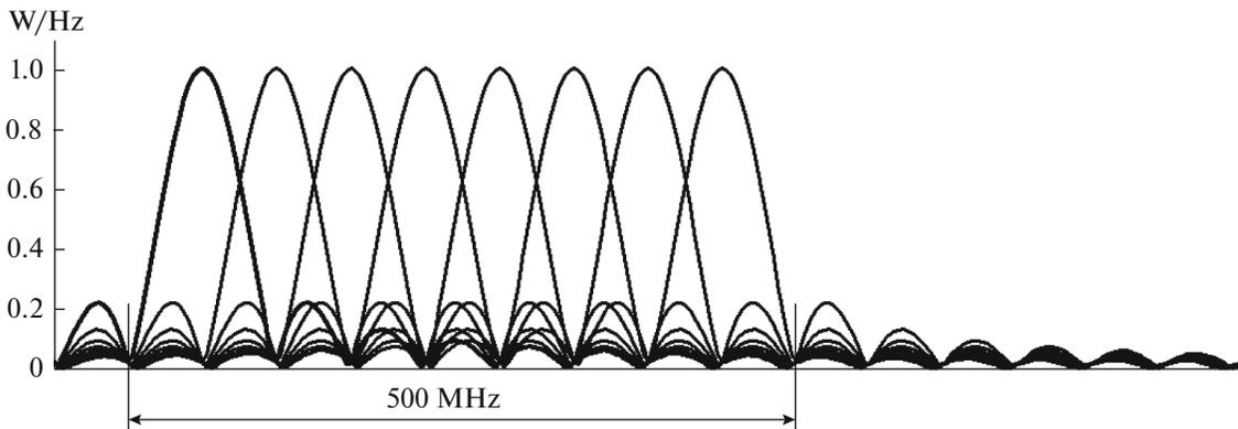
**Fig. 4.** Fragment of magnitudes of spectral density of voltage from eight orthogonal subcarriers.
