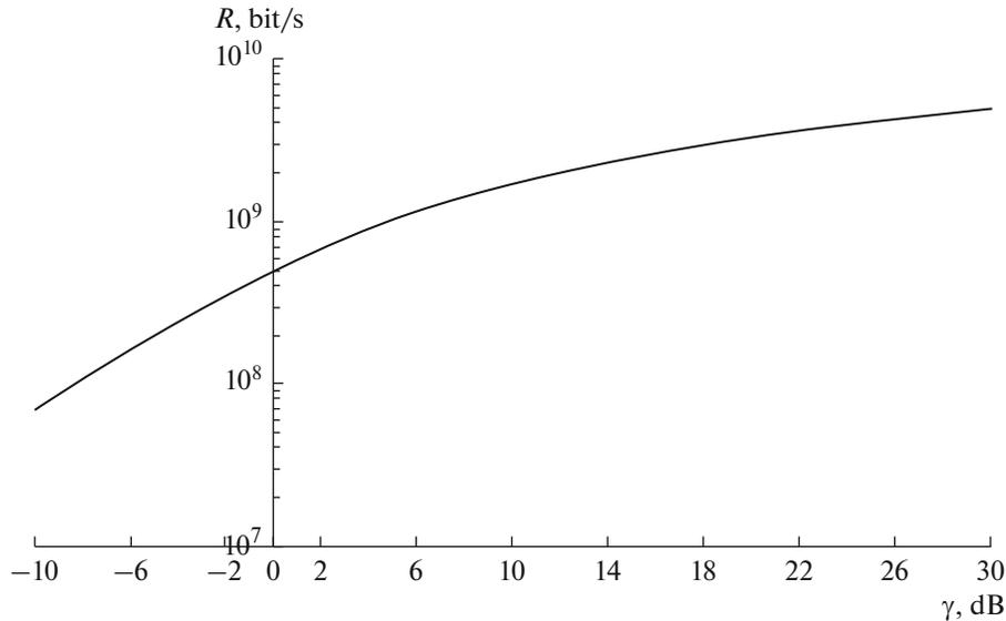
Fig. 1. Dependence of the communication channel transmissivity on the signal-to-noise ratio in channel band of 500 MHz.
