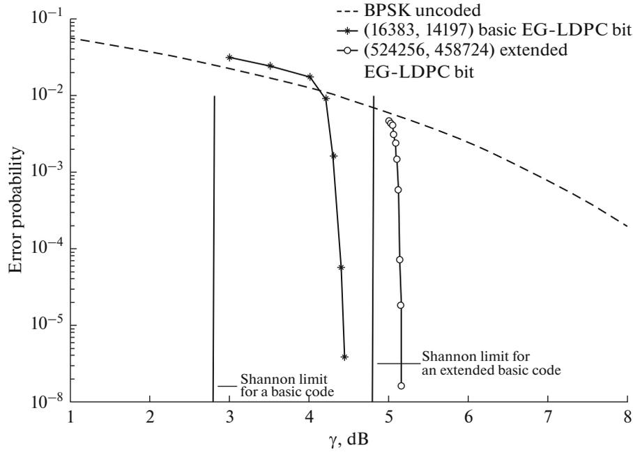
**Fig. 3.** Correcting ability of LDPC codes (16383, 14197) and of extended Euclidean geometric code, LDPC (524256, 507873) with iterative SPA decoding compared with uncoded BPSK signal.
