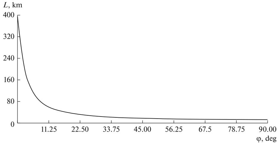
Fig. 6. Dependence of radio signal path length in troposphere depending on antenna elevation angle.
