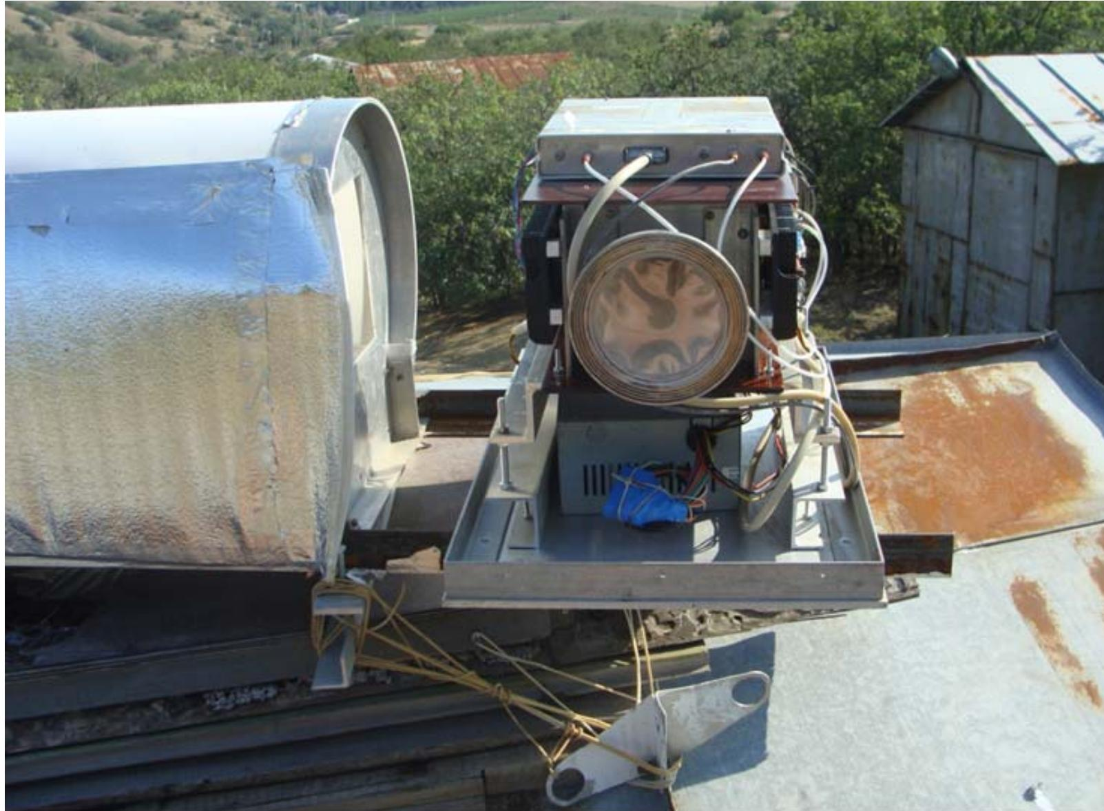
2020-2021. Eight-millimeter radiometer before installation in the working position.
