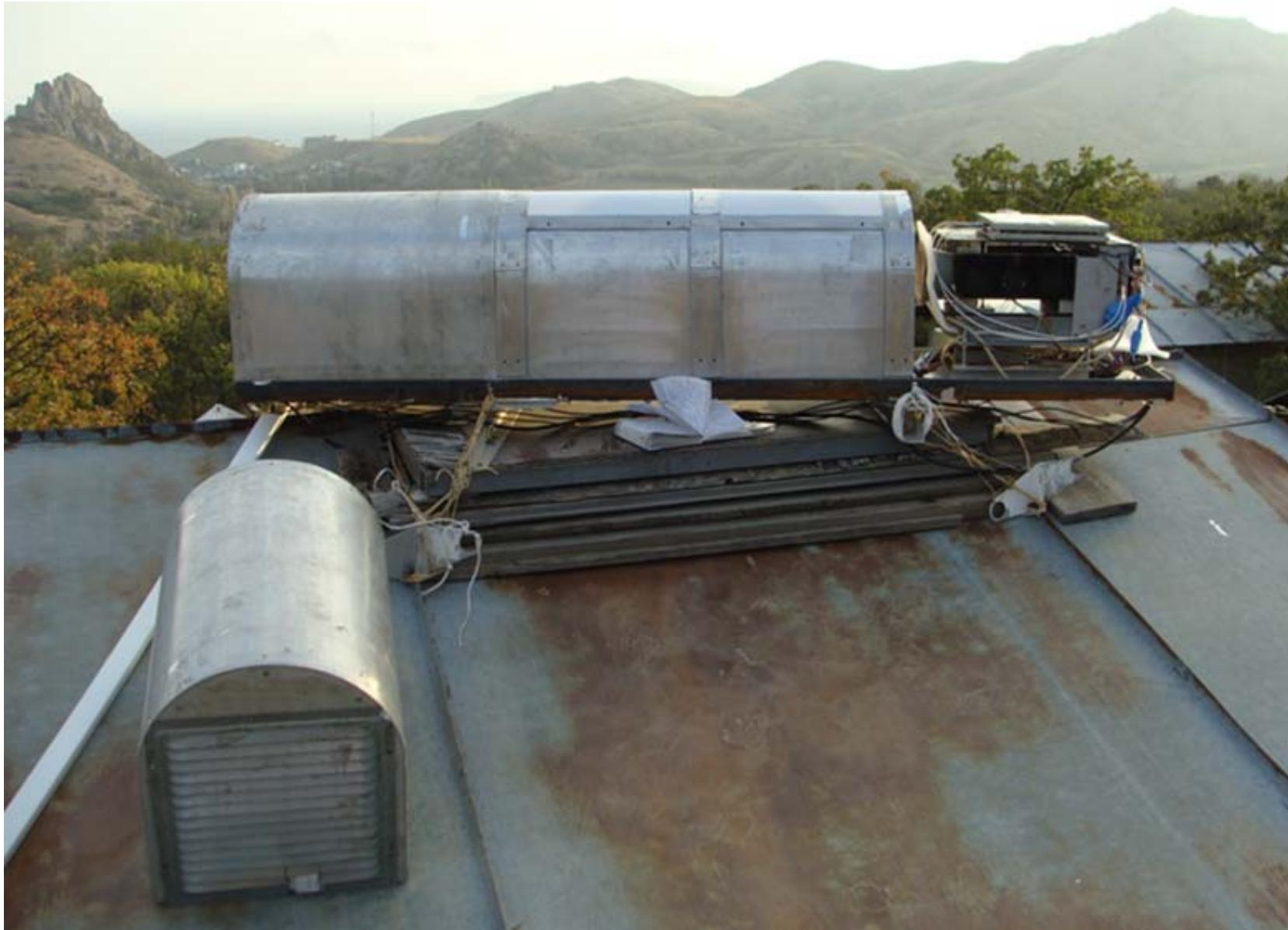
2020-2021. The eight-millimeter radiometer is set to the operating position.
