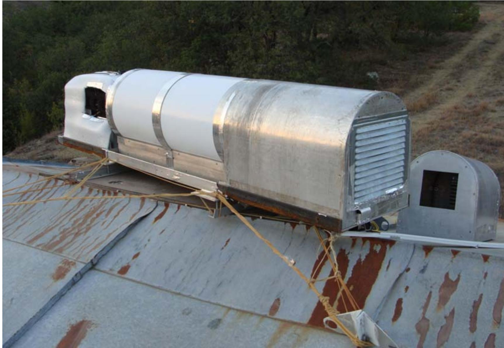
2020-2021. Additional insulation of the eight-millimeter radiometer.
