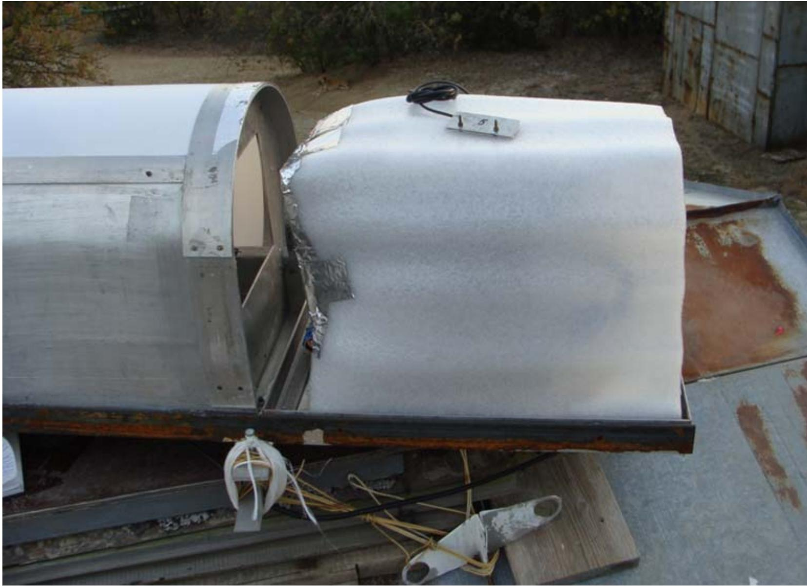
2020-2021. Additional insulation of the eight-millimeter radiometer.
