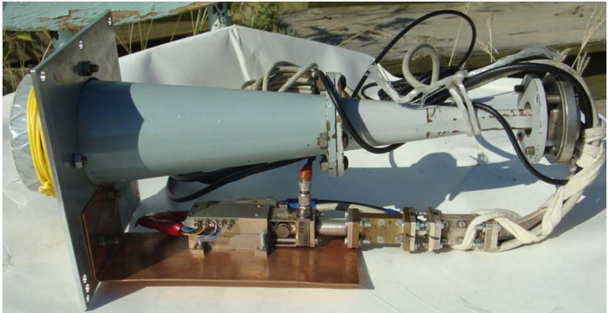
2018. Three-millimeter radiometer without heater and thermoregulation.
