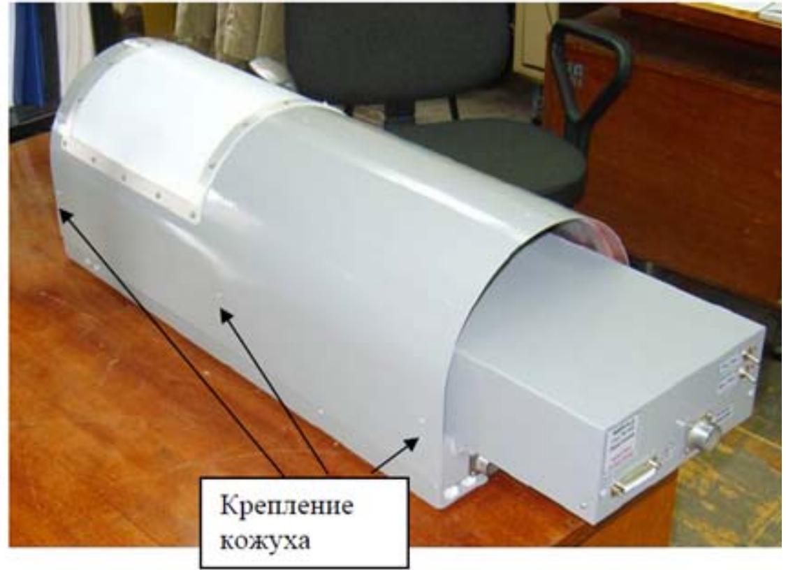
2017. The case of the MIAP-2 device with a transparency window. The surface of the transparency window is not cylindrical.
