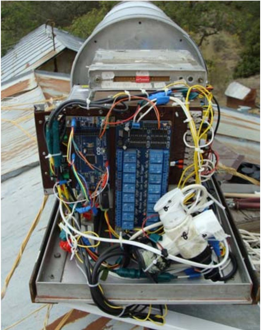
Arduino-based control system for thermoregulation and data transfer from radiometers to the computer.
