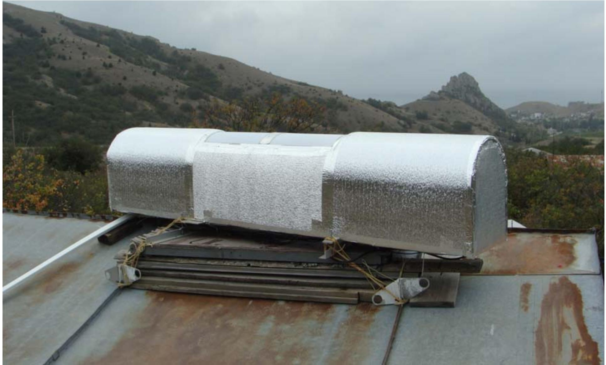
2020-2021 Device in insulation with a thickness of 10 mm. Reverse side.
