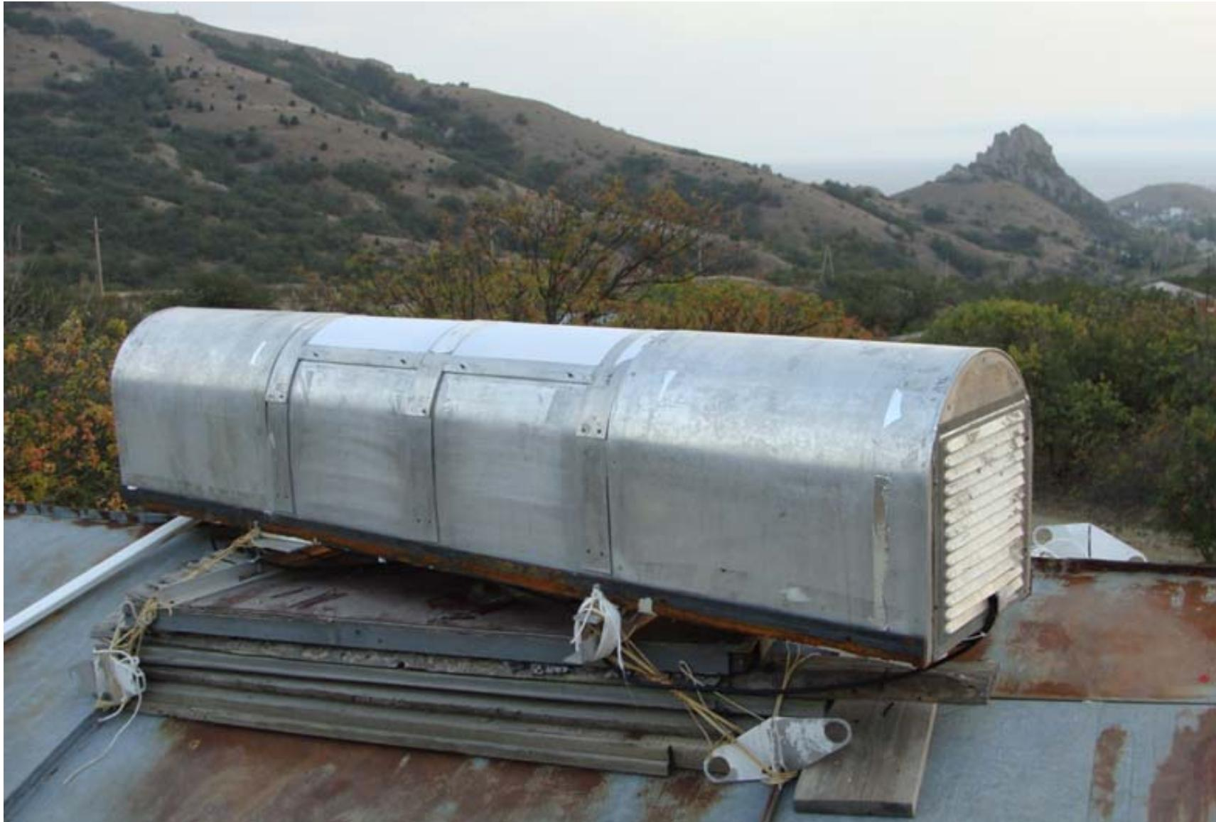
2020-2021. The device is without insulation. The reverse side. Air passes through the side ventilation grilles.
