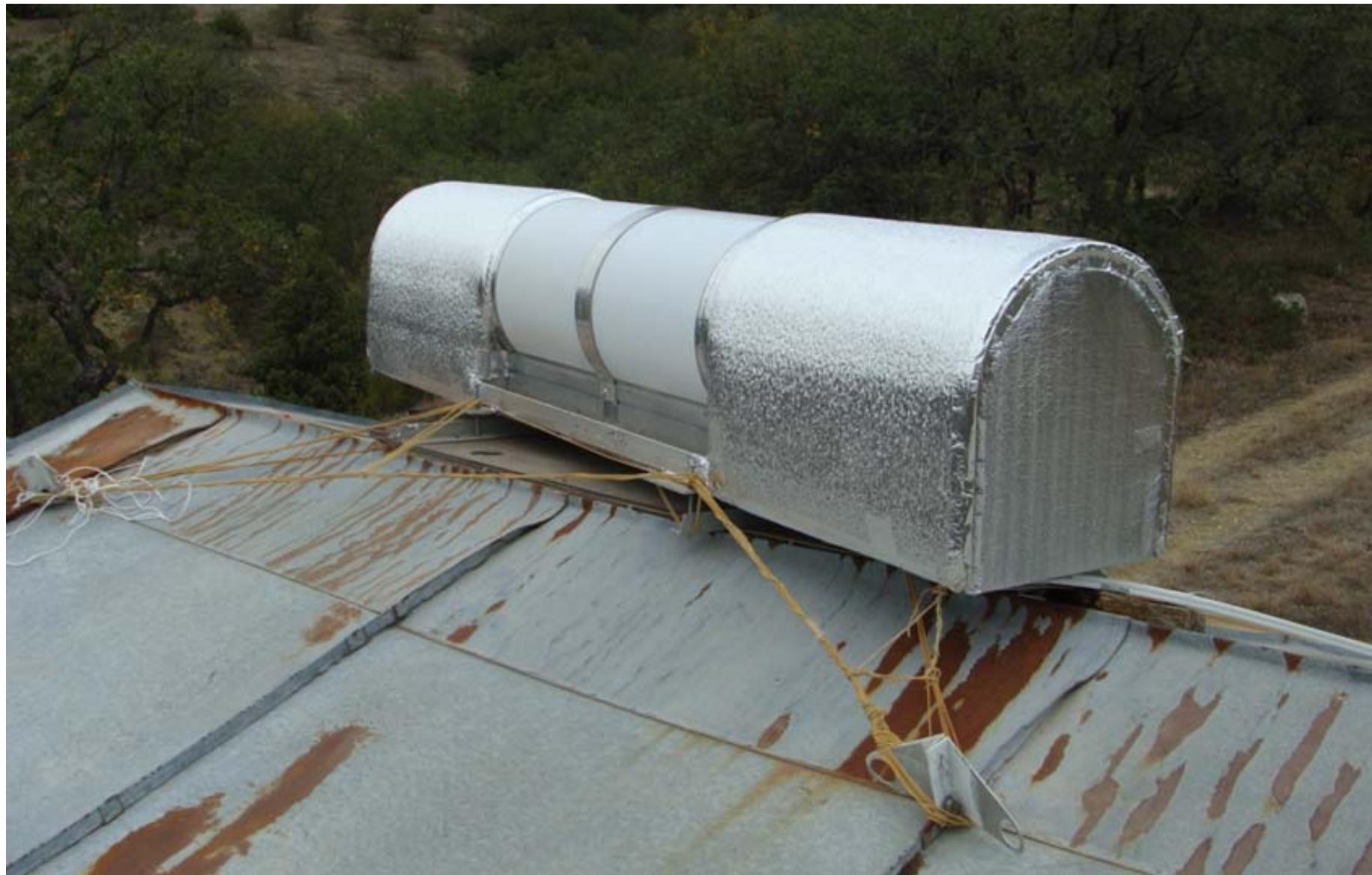
2020-2021. Device in insulation with a thickness of 10 mm. View from the facade. The air inside passes along the sides from below.
