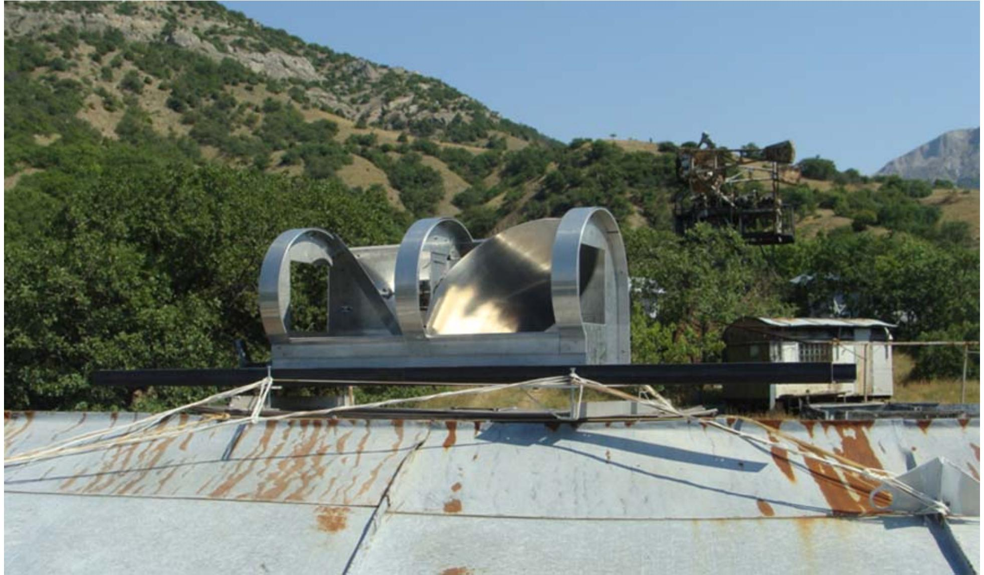
2019. The basis of the device is a rotary module on the corners with adjustment screws. Boxes with radiometers are placed on the left and right corners.
