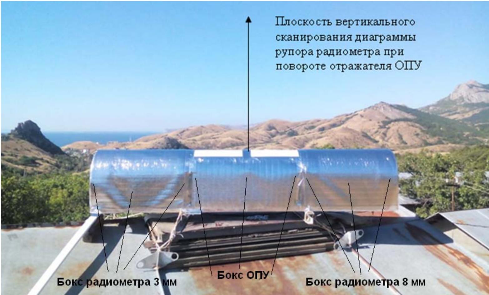
2019-2020. The direction of the scanning plane and the location of the device boxes: Radiometer 3 mm-on the left, Radiometer 8 mm-on the right, Rotary device-in the center. Device in insulation with a thickness of 4 mm. In the distance, near the horizon, the hilltops act as a Black Body.
