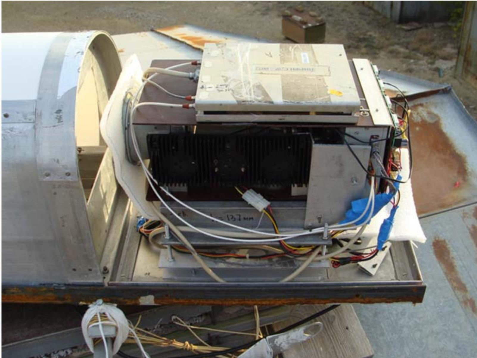
2020-2021. Additional insulation of the eight-millimeter radiometer.
