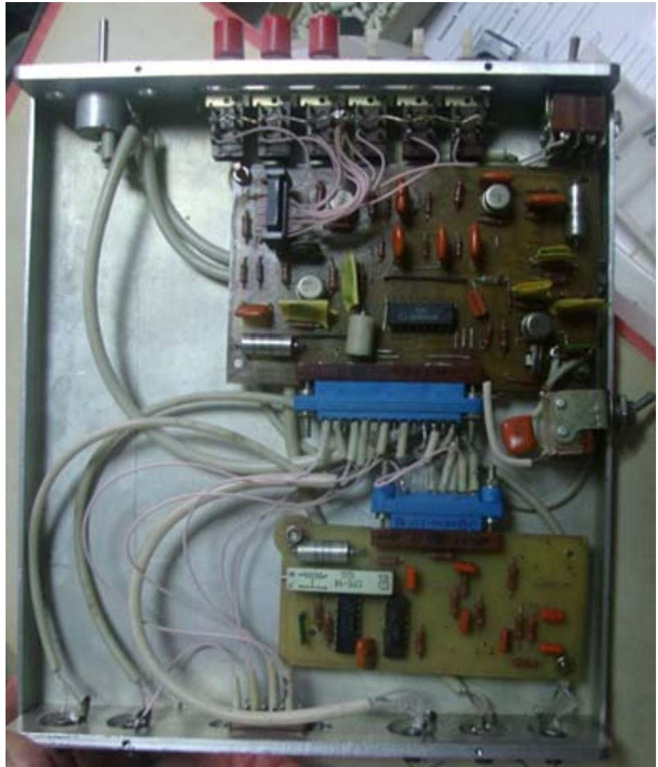
2020-2021. Synchronous detector and reference voltage generator boards.
