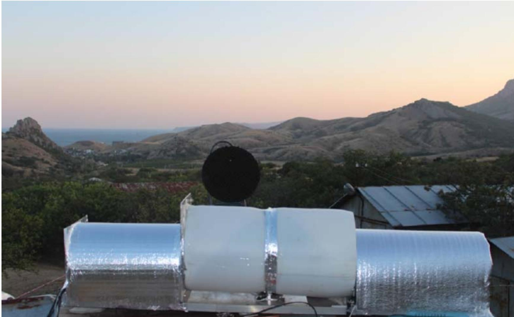
2018. Measurement of the emissivity of the mountain top by the emissivity equal to 1 of the Blackbody disk.
