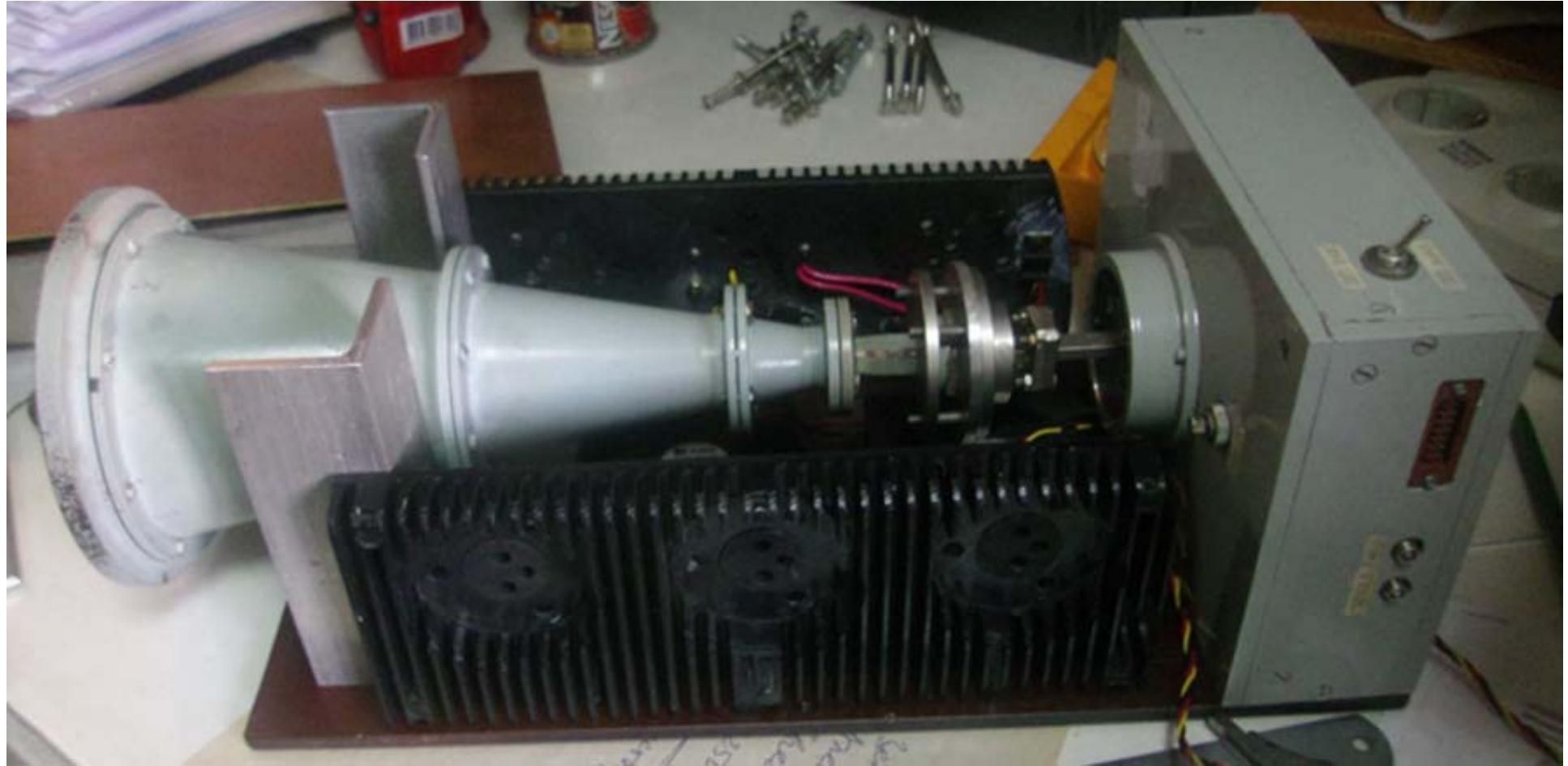
2020-2021. An eight-millimeter radiometer with a working band of 33-35 GHz. The horn is connected to a microwave unit, flanked by two radiators with 12 W heating elements for two temperature controllers.
