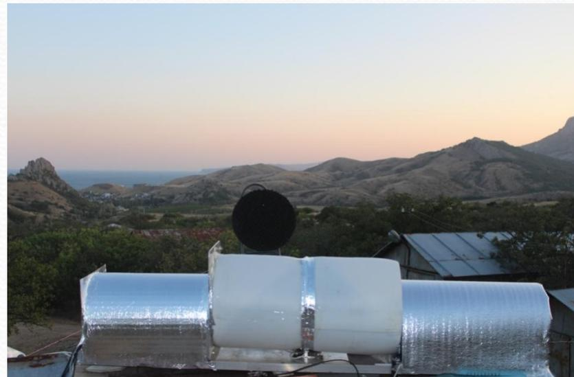
Image of the assembly and preliminary testing of the 3mm channel of the radiometer
