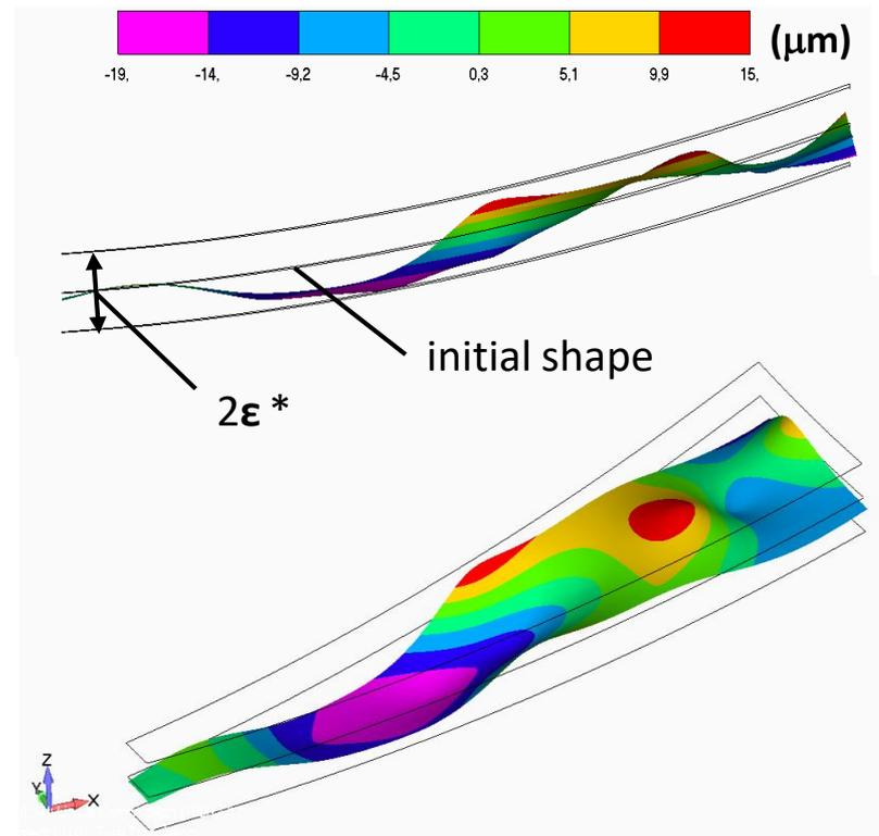
Surface deformation map of the panel at 120 K
