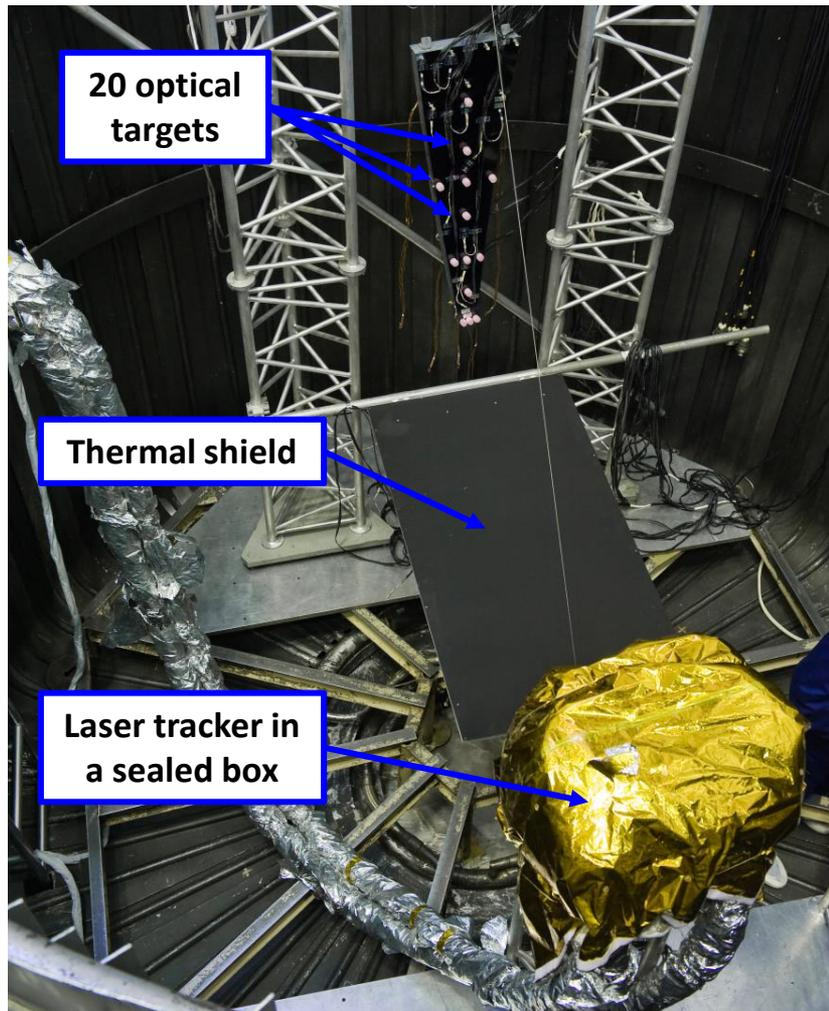
Setup for measurement of thermal distortions of the panel in a thermal vacuum chamber
