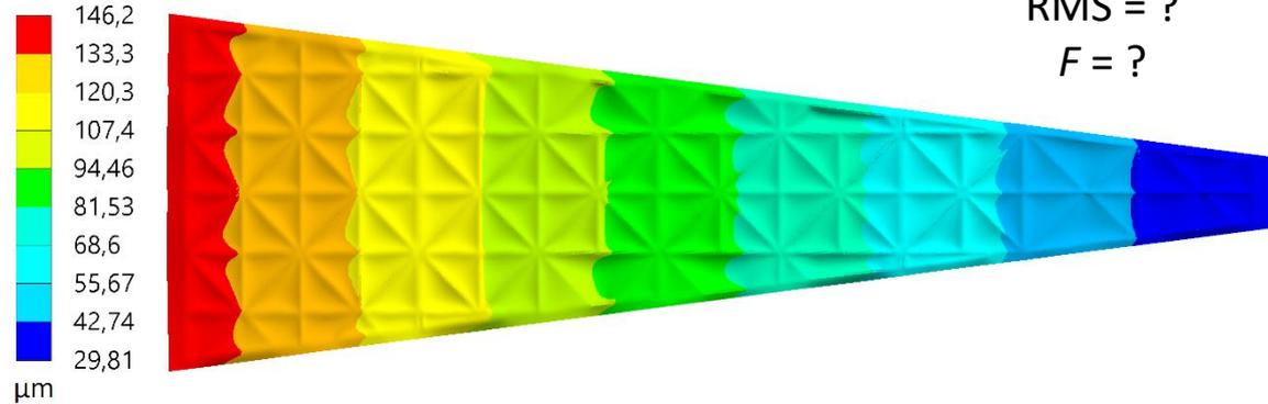
Surface deformation map after cooling down to operational temperature (4.5 K)
