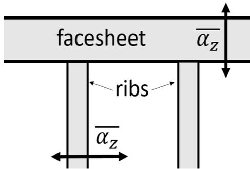
$$\begin{aligned} \overline{\alpha_x} &= \overline{\alpha_y} = 0.3 \cdot 10^{-6} \text{ 1/K} \\ \overline{\alpha_z} &= 25 \cdot 10^{-6} \text{ 1/K} \\ \overline{\alpha_z} &\approx \mathbf{83 \overline{\alpha_x}} \end{aligned}$$
