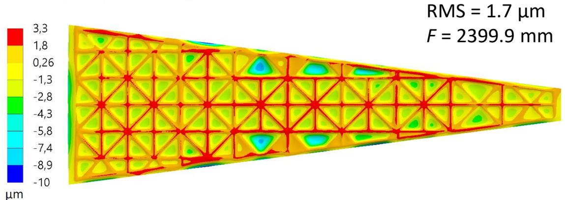
Surface deformation map related to the best-fit paraboloid after cooling down to operational temperature (4.5 K)
