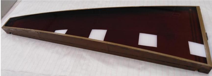
Trial parabolic mold from ULE glass
