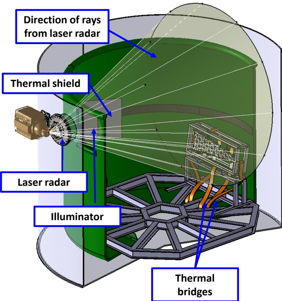
Setup for measurement of thermal distortions of the panel in a thermal vacuum chamber
